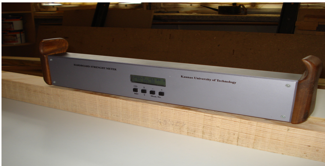
Fig. 7. Stiffness-strength estimation and defect inspection
